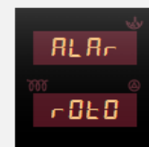
Alarm Burnig pot rotation failure
