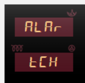
Alarm Thermocouple in the Chamber
